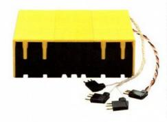
The four-channel motor controller has two analog channels (speed/direction controller) and two digital channels (relays).
